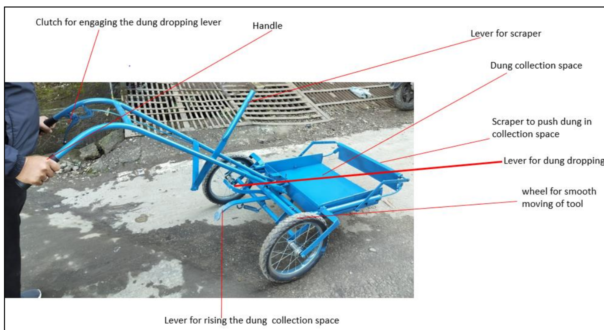
Fig 3: Developed Manual dung scraper prototype
